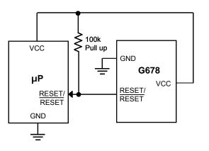
ICC may increased at high  $T_A$ , Therefore, can not connect Resistors to VCC to prevent lcc abnormal behavior at high  $T_A$ .
