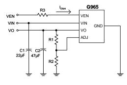
$VO = \frac{1.2 \; (R1+R2)}{R2} \quad Volts$   $R2=12k\Omega \; is \; recommended$   $R3 \; should \; be \; connected \; for \; current \; I_{ENH}$   $restriction \; as \; V_{EN} > V_{IN} + 0.3V$   $R2=0\Omega \; sets \; V_0 \; to \; fixed \; output \; mode.$
